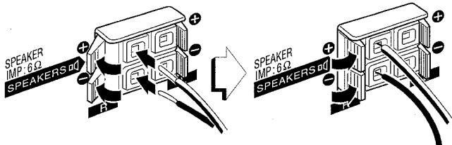
The speaker cord with the white stripe should be connected to the **+** terminal and the black cord to the **-** terminal.
